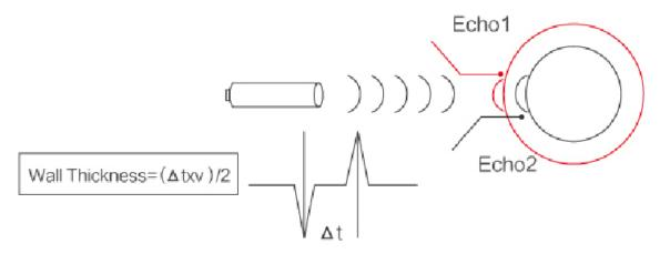
$\triangle \mathbf{t}$ = The interval time between the two waves
